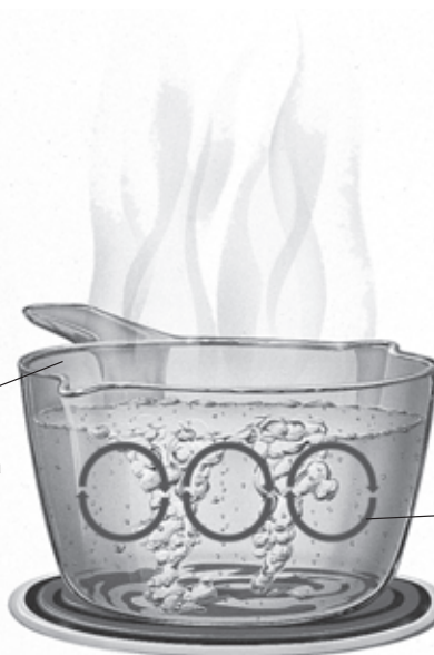
The repeated rising and sinking of water during boiling are due to convection.
