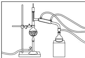
**Distillation** is the process that separates a mixture based on boiling points. Water in this mixture evaporates and then condenses as pure water.
