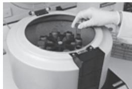
Blood is separated into its parts by a machine called a **centrifuge**. In the test tube of blood above, a layer of plasma rests atop a layer of red blood cells. A centrifuge separates mixtures by the densities of the components.
