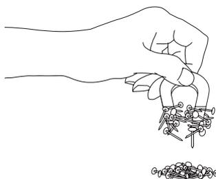
A **magnet** can be used to separate a mixture of the elements iron and aluminum. Iron is attracted to the magnet, but the aluminum is not.
