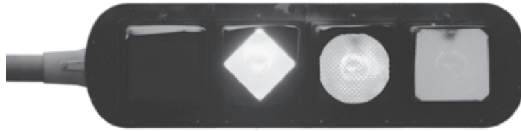
This stoplight in Canada was made to help the colorblind see signals easily.
